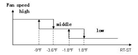
2.2.4.7 Pre-heat control: After selecting heating mode, when IPT≥100.4°F, indoor fan motor will run according to the setting. When IPT<100.4°F, indoor fan motor will delay starting until compressor runs for 60 seconds.
