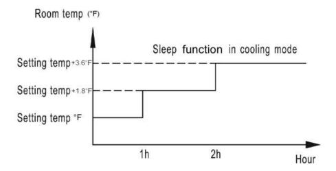
2.2.8.3 In heating mode, at the beginning of sleep function, if room temperature < setting temperature, the compressor, outdoor fan and four-way valve will start normally. Indoor fan motor will run in low speed. If room temperature ≥ setting temperature, the unit will start sleep mode. Fan speed will be set at low speed. Air flow direction can be adjusted or stay in one position.
