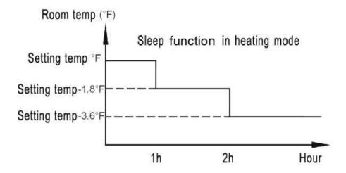
NOTE: When Timer and Sleeping function are set at the same time, the unit will work with Timer function.
