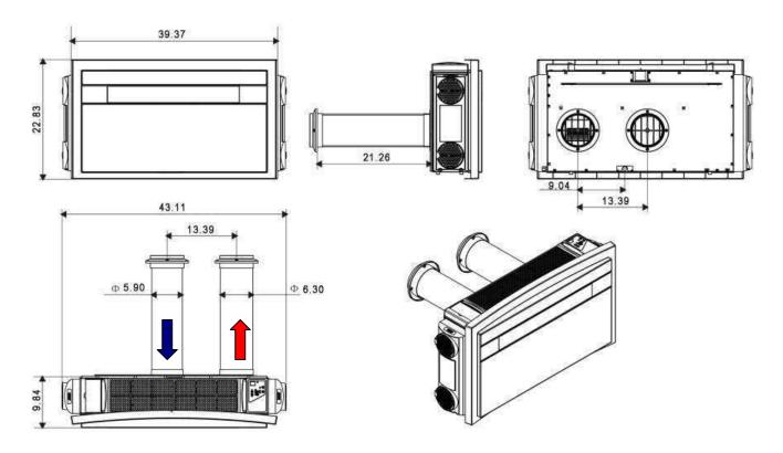
**Note:** The external pipes have two different diameters, use Ø6.30in for air outlet side (see red arrow) and Ø5.90in for air inlet side (see blue arrow).
